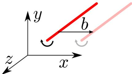
Figure 8: Momentum changes whenever the vortex shifts with respect to the fluid.
