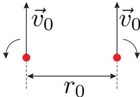
Figure 3: Parallel vortex filaments with opposite circulations
