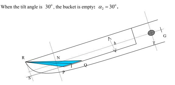
1.3. Determining the tilt angle  $\beta$  of the lever and the amount of water in the bucket m when the total torque  $\mu$  on the lever is equal to zero
