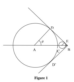
Let us consider a plane containing the particle trajectory. At t = 0, the particle position is at point A. It reaches point B at  $t = t_1$ . According to the Huygens principle, at moment  $0 < t < t_1$ , the radiation emitted at A reaches the circle with a radius equal to AD and the one emitted at C reaches the circle of radius CE. The radii of the spheres are proportional to the distance of their centre to B:
