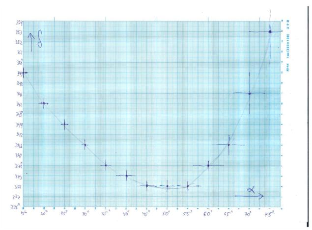
By observing the remote screen, it is possible to identify the point in which  $\delta$  is minimal at the highest accuracy.
