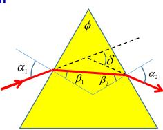
For the symmetric case, the incident angle  $\alpha$  holds the relation  $\alpha = \frac{\delta}{2} + \frac{\phi}{2}$  and from Snell's
