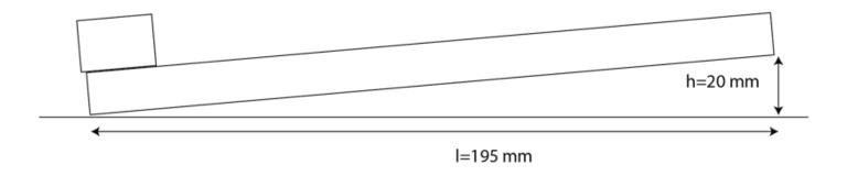
$h=20\pm1$  mm,  $l=195\pm2$  mm. The latter uncertainty is larger due to difficulty lining up ruler with projection of end of the board.
